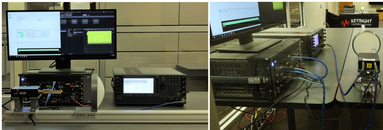
Figure 3. OTA quasi-optic transmission at 285 GHz with 30 GHz bandwidth, transmit side.
