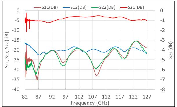
Testing was done at room temperature using a PNA with WR-8 frequency extension modules rated for 90-140 GHz. The ringing below 85 GHz is systemic and not caused by the isolator. Cryogenic tests are coming.
