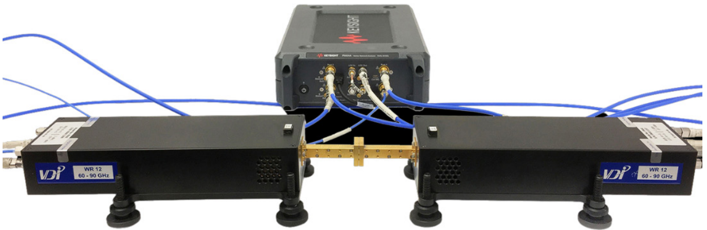
Figure 1: VNA extenders can now be used with new streamlined USB VNA devices that are smaller, portable and cost much less than the benchtop models - extending test capabilities up to 400GHz
