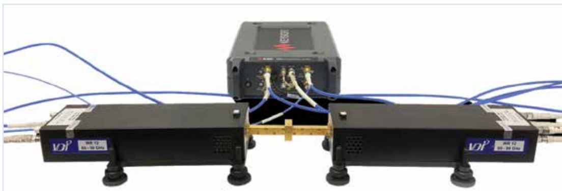
Figure 2: Virginia Diodes VNA extenders can now be used with new streamlined USB VNA devices that are smaller, portable and cost much less than the benchtop models, extending the test and measurement capabilities up to 400 GHz.
