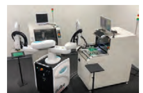
Automation of PCB loading & unloading
